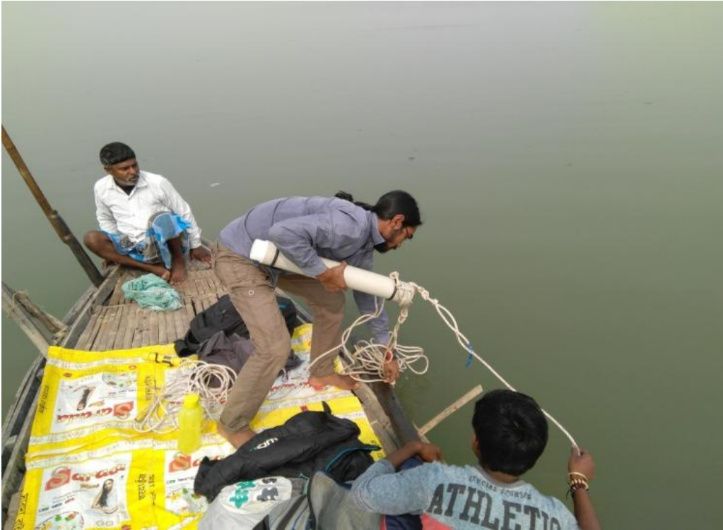
A CPOD being deployed from a moored fishing boat in Barari with weights attached. The device logs dolphin clicks but does not record their sound.
