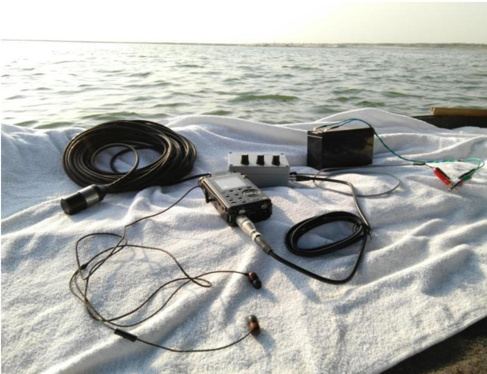
The hydrophone set used to record dolphin sounds and noise from motorised vessels in the river.
